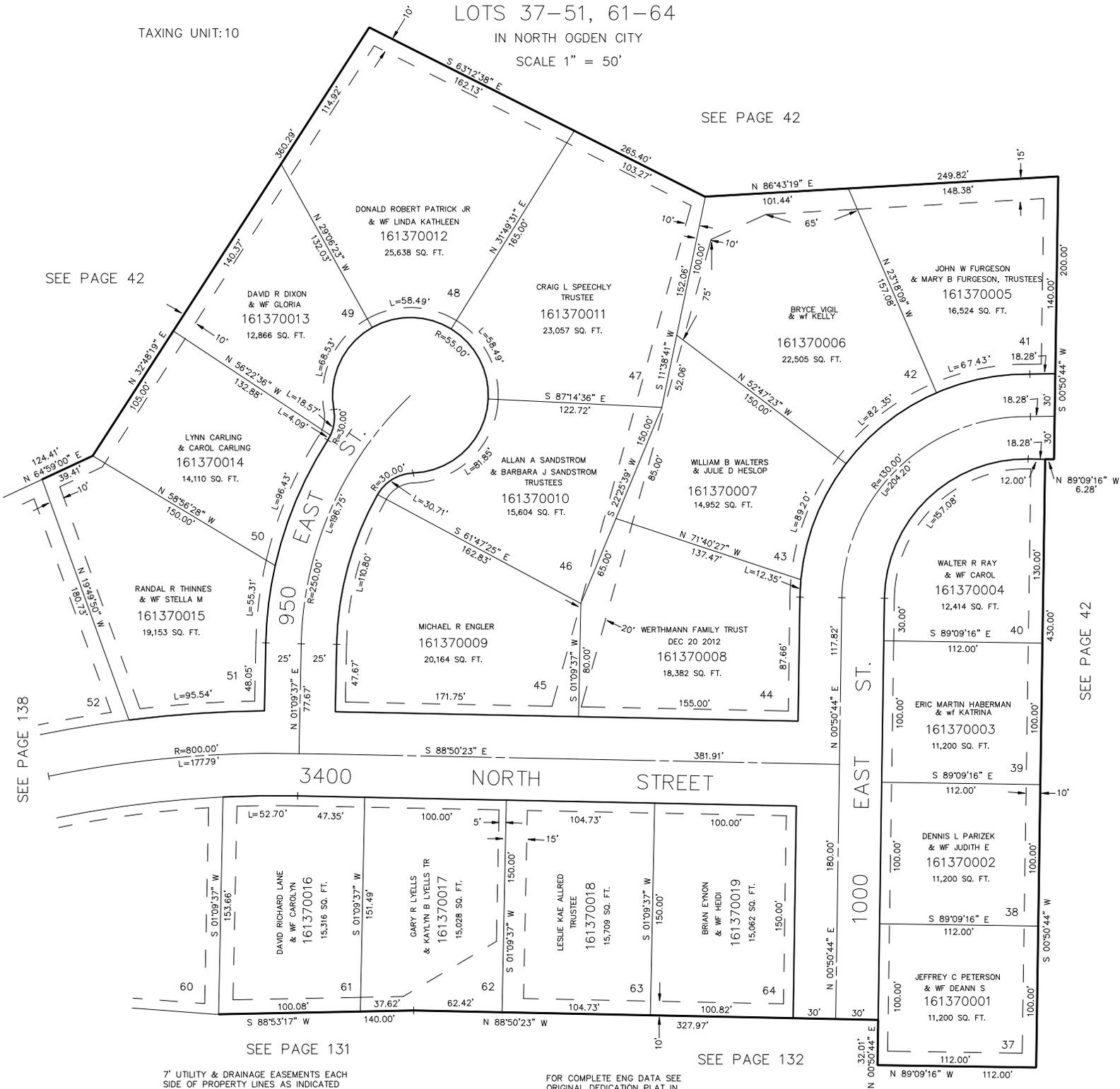
7' UTILITY & DRAINAGE EASEMENTS EACH SIDE OF PROPERTY LINES AS INDICATED BY DASHED LINES EXCEPT AS OTHERWISE SHOWN.
